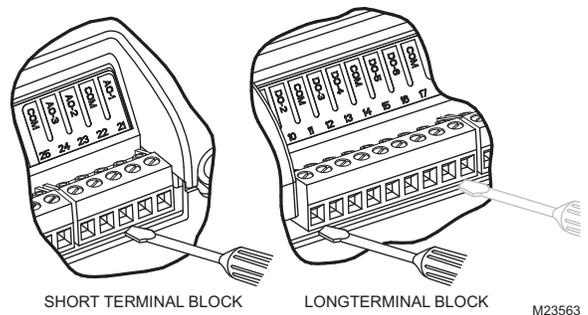
**Fig. 25. Removing Terminal Blocks.**
