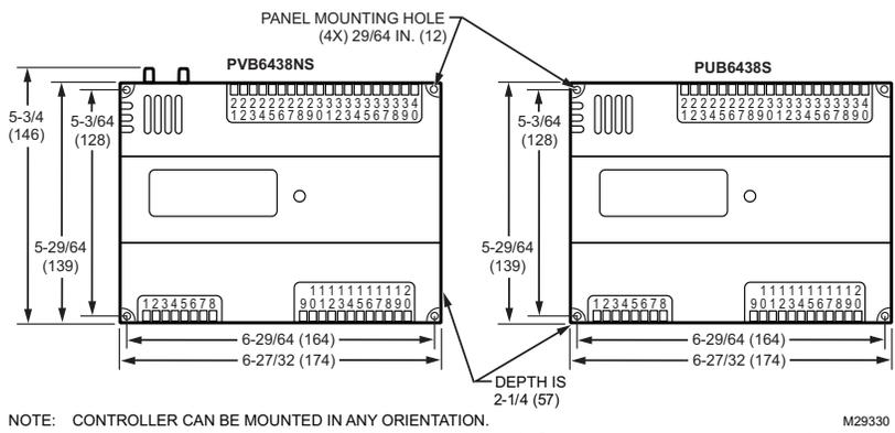
**Fig. 7. Panel mounting - controller dimensions in inches (mm) for models PUB6438S, PVB6438NS and PUB6438SR.**
